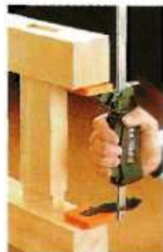
Simply reversing the jaws on the E-Z Hold clamp allows you to use it as a spreader.
