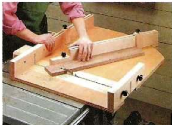
Angled Cuts. By attaching an adjustable fence that pivots around the curved end of the sliding table, you can make angled cuts as well.
