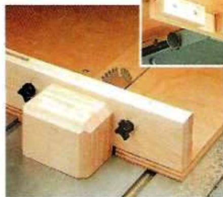
C. Safety System. A thick wood block and two stops prevent the blade from being exposed at the end of a cut.
