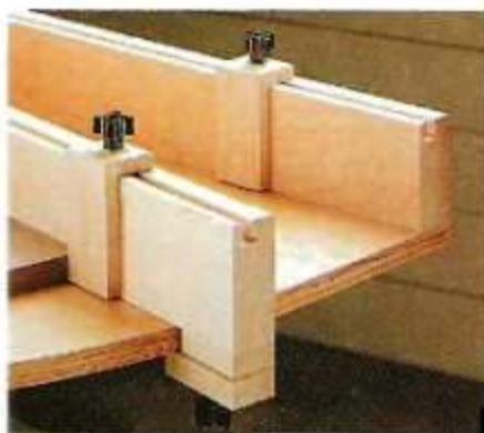
A. Stop Blocks. A pair of stop blocks allows you to cut multiple pieces to length quickly and accurately.
