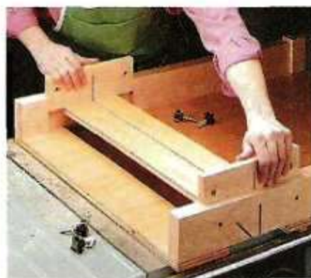
B. Inserts. Two removeable inserts (one for 90° and the other for 45° cuts) reduce chipout on the bottom of a workpiece.
