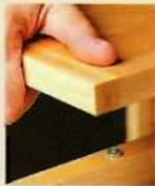
A dowel center makes it easy to locate the hole for the steel pin in the bottom of the work table.
