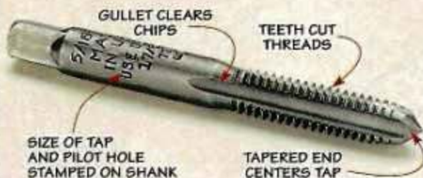
▲ A tap is specially designed to cut threads inside a hole. They're sold individually (like a drill bit) or as part of a tap and die set at most hardware stores.
