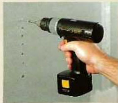
C. Clutch. Screwing sheetrock to wall studs gave us a feel for how well we could fine tune the clutch.
