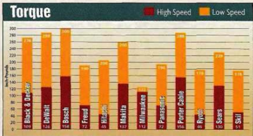
D. Torque. Finally, we used a torque wrench to measure the torque at high and low speed.
