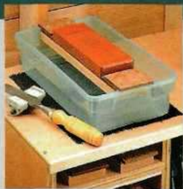
▲ Spanning a plastic container filled with water, a simple holder anchors the sharpening stone.
