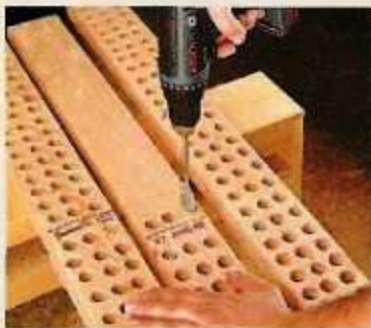
A. Drilling. To test how much "gas" these drills had, we drilled \frac{3}{4} "-diameter holes in Douglas fir.
