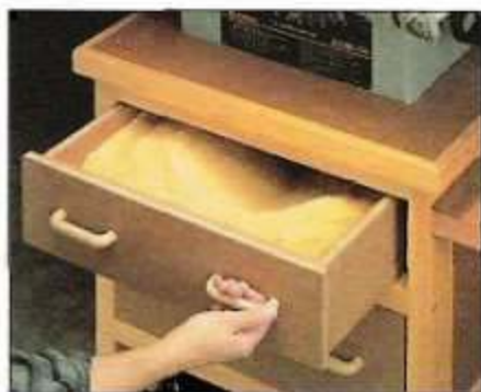
B. Dust Bin. A bin below the saw cabinet collects dust. When it’s full, the bin pulls out for easy emptying.
