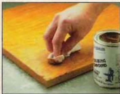
Step 4. To get an even shinier finish, apply a polishing compound in a circular motion. Then buff it out when dry.
