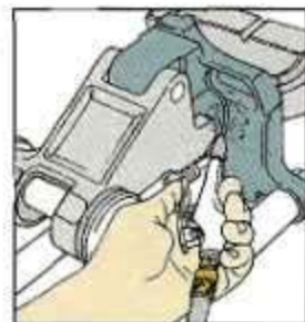
Clean Saw. To clean a table saw, the first step is to blow away any trapped sawdust from inside the saw cabinet. Then scrub away the pitch and resin build-up.
