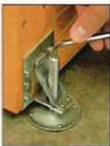
An Allen wrench is all that's needed to adjust these heavy-duty levelers and raise the cabinet off its casters.
