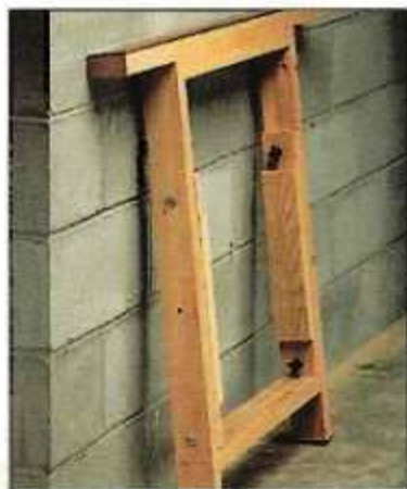
▲ Storage. For compact storage, tuck the arms that connect the outfeed support to the cabinet inside the frame and tighten the knobs.
