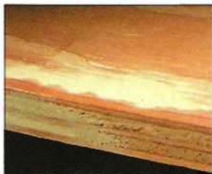
B. Filler. Small knots, gaps, and minor surface imperfections are generally filled with a synthetic wood filler.
