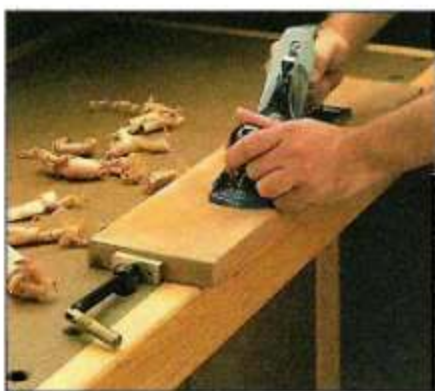
B. Bench Dog. A hex bolt (photo A) and a Veritas Wonder Dog make a functional bench dog system.
