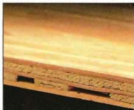
C. Voids. In addition to the face veneers, you can get a feel for the quality of the plywood by checking for voids.
