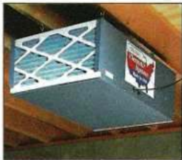
Suspended Filter. If floor space is a premium, consider a filter unit that can be suspended overhead.
