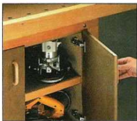
C. Cabinet. The cabinet is a convenient place to store hand tools. It also adds extra mass to the workbench.
