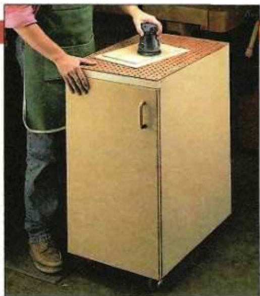
▲ This shop-built sanding table pulls in the dust that's produced when sanding. And it doubles as an air filter system for your shop.
