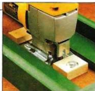
▲ In addition to cleats that keep the saw from moving side to side, two wood blocks lock it in place.
