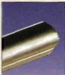
Because of its fingernail shape, a spindle gouge doesn't have any corners to "catch" the workpiece.
