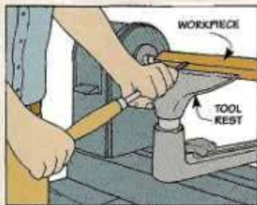
Step 1. With your hand against the tool rest, wrap your fingers around the blade in an overhand grip.
