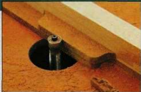
Identical Parts. A quick way to produce identical parts is to make a template and use it as a pattern for a flush trim bit to follow.
