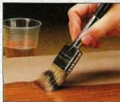
A. Flow On. Hold the brush at about a 45° angle to the workpiece and flow on a heavy coat of varnish.
