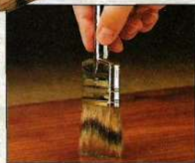
B. Tip Off. Now hold the brush upright and use the tips of the bristles to remove any brush marks.
