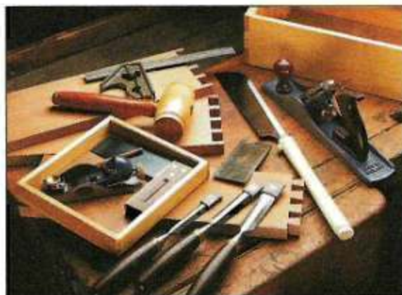
Hand Tools. A chisel set, a few hand planes, and a square or two are just a few of the hand tools that should be in every woodworking shop.
