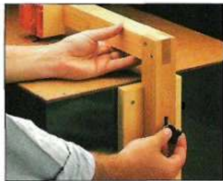
C. Adjustable Arm. The arm that supports the guide system and hold-down adjusts for different thicknesses of stock.
