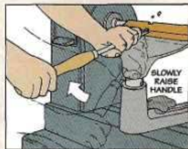
Step 2. Starting with the handle of the gouge down low, gradually lift up on it to produce a shaving.
