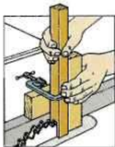
A safe way to cut an open mortise on a long workpiece is to clamp it to a support jig that's made by screwing scraps of 2x4 together.
