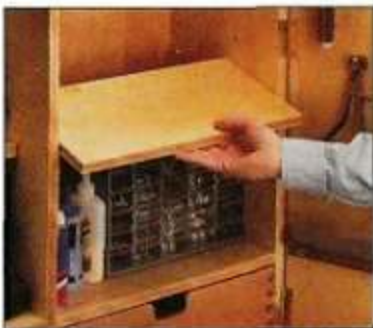
B. Shelves. Adjustable shelves provide additional storage. And they stay put when removing a tool.
