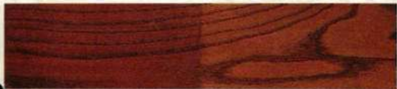
B. Dark or Light. Although it can obscure the grain of the wood a bit, leaving some of the excess stain on the board creates a dark color (left). To produce a lighter color, just wipe the board "dry" (right).
