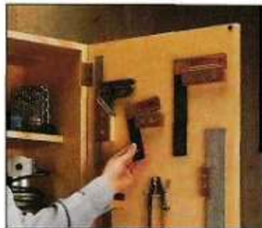
A. Tool Holders. Hand tools hang on special, shop-built holders to help protect them from damage.
