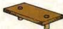
A scrap piece of Masonite with dowels fits into the pegboard to act as a simple cleat.
