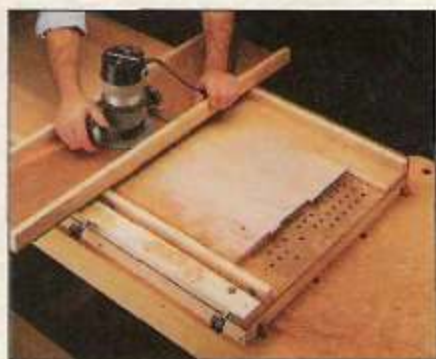
B. Wide Panels. The thicknessing jig can handle glued-up panels and wide boards up to 15\frac{3}{4} " in width.
