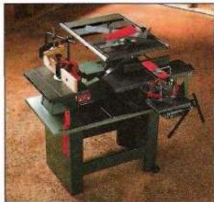
▲ A multipurpose tool such as this Kity K-5 combines a table saw, edge jointer, thickness planer, shaper, and mortiser. It has many of the advantages that similar stationary tools have, but takes less space. (Farris Machinery; 800-872-5489)
