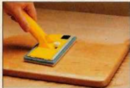
C. Pad. For large surfaces, a paint pad works best. It loads well and lets you apply the finish quickly and evenly.
