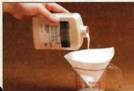
A. Filter. To strain out any lumps in the finish, pour it through a paper paint filter into a plastic (or glass) container.
