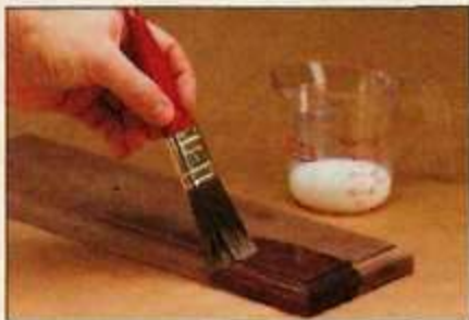
B. Brush. A synthetic bristle brush (nylon or polyester) helps lay down a smooth coat of finish on small pieces.
