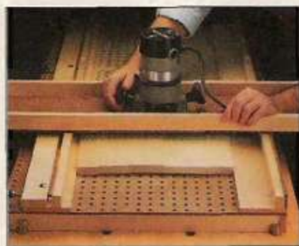
C. Flattening. In addition to smoothing stock, this jig can also flatten a cupped or warped workpiece.
