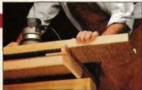
▲ Grooves in the bottom of the carriage fit over the carriage guide on the platform to produce overlapping passes.
