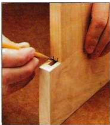
Thickness. To establish the thickness of the tenon, draw lines just inside the walls of the mortise.
