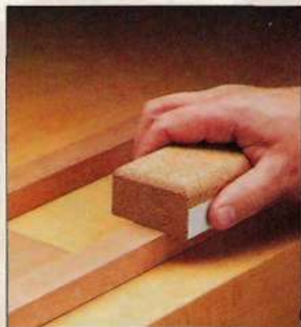
C. Hand Sanding. But on a narrow workpiece, a sanding block ensures a crisp corner and a flat surface.
