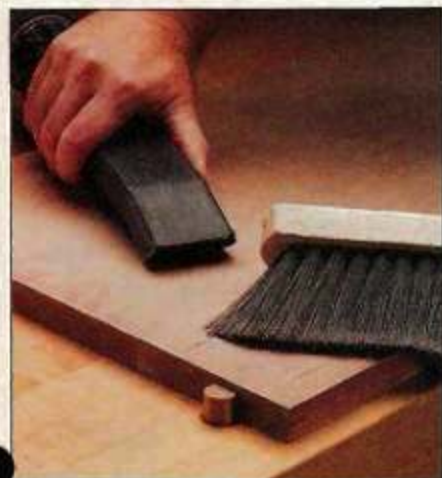
D. Vacuum. Remove sanding dust and bits of abrasive that have fallen off with a shop vacuum and brush.
