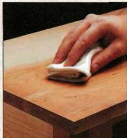
F. Mineral Spirits. Wiping down the surface with a rag soaked in mineral spirits reveals stray glue smudges.
