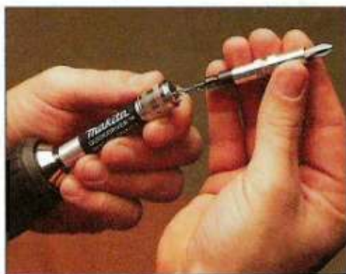
Combination Tool. For fast assembly, this system has a special holder that houses one bit while you're using the other one.
