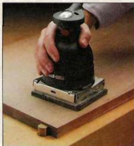
B. Power Sanding. A power sander makes quick work of removing material on large, flat surfaces.
