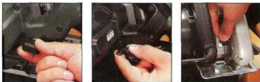
Depth Adjustment. The plastic knob on the Quantum (left) provides a more comfortable grip than the wing nut on the B&D (center). But neither are knuckle-busters like the depth adjustment lever on the Skil (right).
