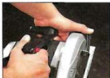
Blade Guards. The compact design of the Skil (left) lets you retract the blade guard and grasp
