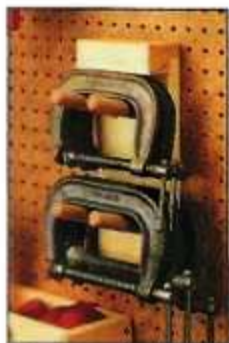
The wood pegs on this hanger make it easy to slip your C-clamps on or off.
