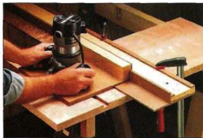
Router. With the cutting guide clamped across a wide panel, it can also be used to turn your hand-held router into a precision tool when routing dados (or grooves).
