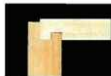
Bit is too low.
