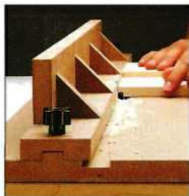
Back. Because the groove that fits over the key is offset, the back of the fence allows you to cut a rabbet on the end of a workpiece.
