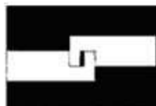
Fence is too close to bit.
