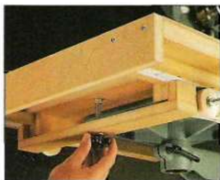
C. Fence Brake. Once the fence is adjusted where you want it, lock it in place by tightening the knob on the brake.
