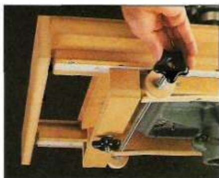
B. Micro Adjuster. A mechanism underneath the table allows you to micro-adjust the fence to fine tune the position.
