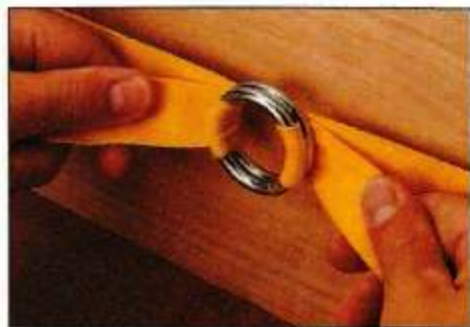
▲ With the wing nut on the clamp backed off all the way, slip the band around the project and tug the ends to remove the slack.
