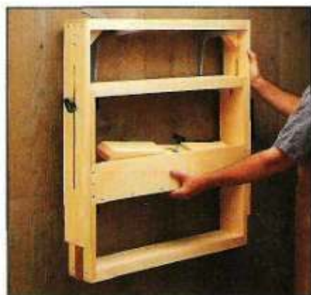
C. Compact Storage. When it’s not in use, you can knock down the sawhorse and store the feet in the tray.
