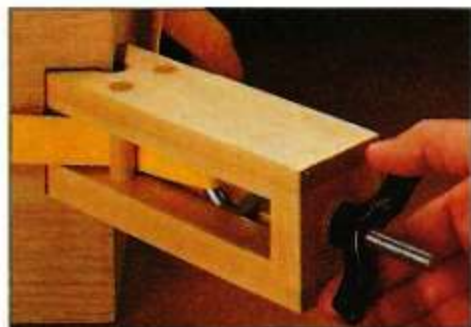
▲ Now fit the jaws of the clamp on a corner of the project, reposition the strap (if necessary), and tighten the wing nut.
