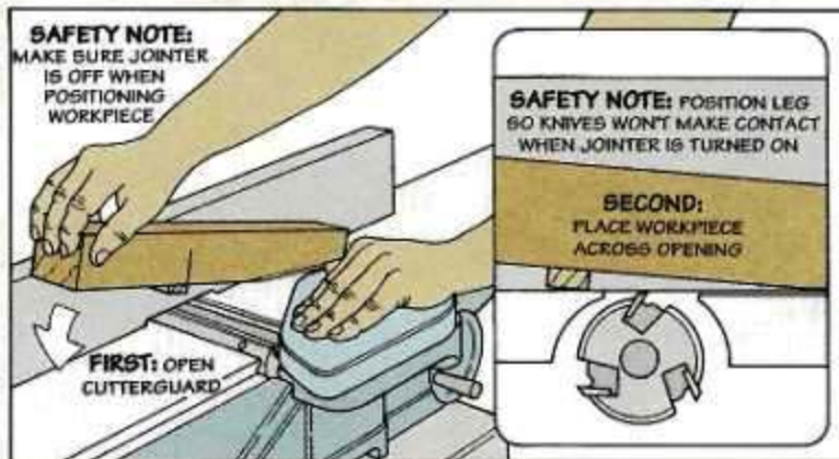
Step 5: With the jointer turned off, open the cutterguard and place the leg on the table so it straddles the opening. Then check that the knives won't contact the leg when the jointer is turned on.
