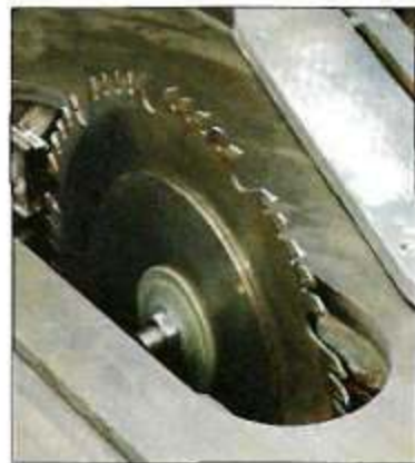
▲ Stabilizer. By adding side support, a stabilizer dampens noise produced by a wobbly blade.
