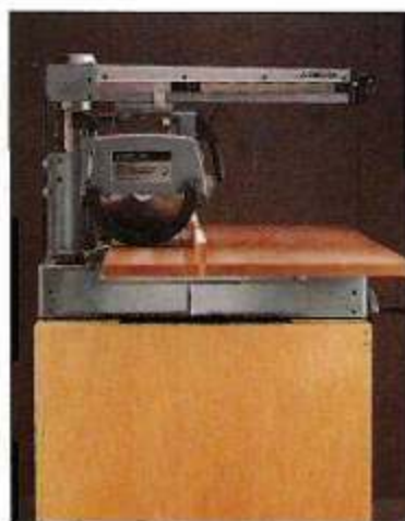
▲ If you have a saw with a long frame, it may not be necessary for you to angle the front for the height adjustment handle.
