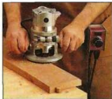
▲ Speed Control. To reduce the RPM's (and noise) of a fixed speed router, use a speed control unit.
