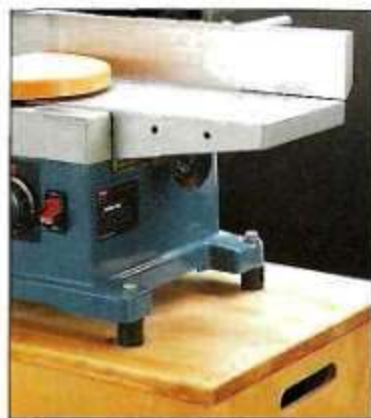
▲ Isolation Mounts. Hard rubber cylinders "isolate" the vibration set up by the motor on a tool.
