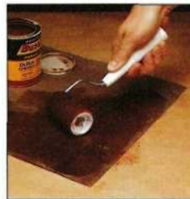
Step 2. Next, you can apply one or two coats of contact cement to the paper-backed side of the veneer.
