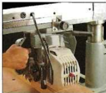
▲ Induction Motor. A heavy motor housing and slower speed contribute to a quieter running tool.
