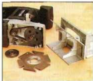
▲ Belt-Driven. A belt-driven tool offers a quieter method of getting power from the motor to the blade.
