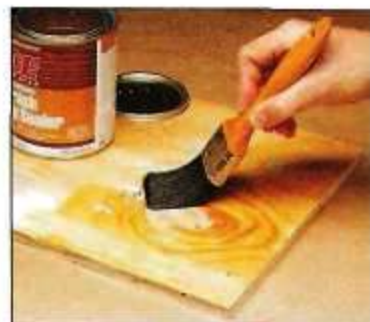
Step 2. To help the contact cement stick, seal the surface with a thin coat of sanding sealer.
