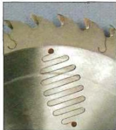
▲ Quiet Blade. Slots and sound-absorbing plugs reduce the noise level of this blade from 92 to 88 dB.
