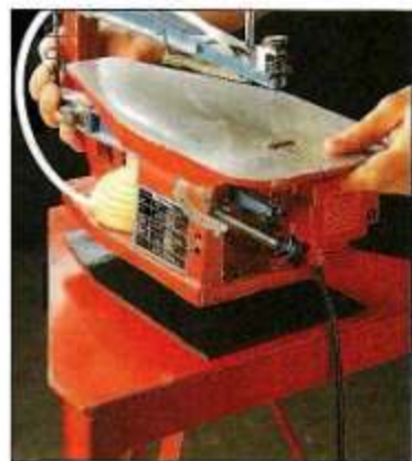
▲ Anti-Vibration Pad. This rubber-like pad absorbs vibration instead of transferring it to the stand.
