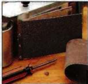
A graphite platen helps reduce heat build-up and extends the life of your belts.
