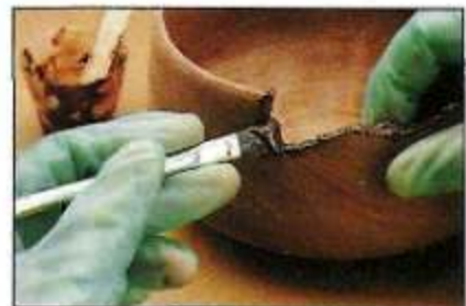
Step 3: Apply the thickened mixture to one surface only. Then bring the parts together and allow to cure.
