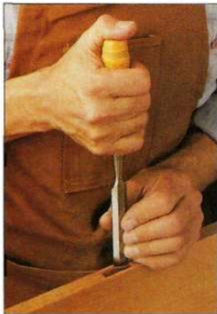
B. Overhand Grip. When making a vertical cut, an overhand grip lets you pare straight down. To help guide the blade, hold it loosely between your fingers.
