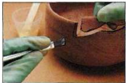
Step 1: Mix the resin and hardener together thoroughly and apply a coat to both surfaces to be joined.
