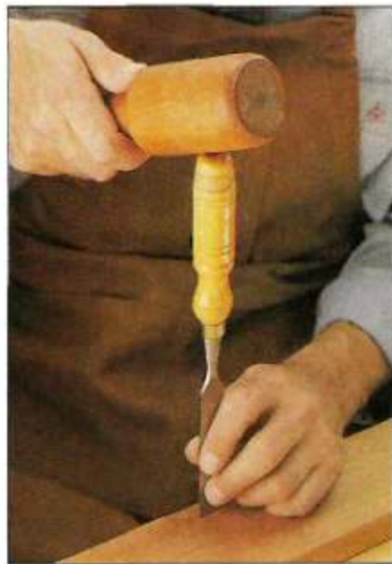
C. Blade Grip. Holding the blade of the chisel lets you pinpoint where the cutting edge enters the work. This is especially handy when using a mallet.
