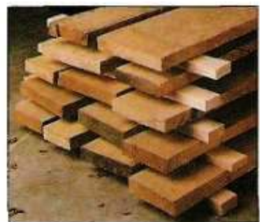
Stacking the boards with small strips in between allows the wood to adjust to the moisture level of the air in the shop.
