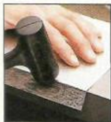
To create a sharp corner, bend the metal over the edge of your saw table with a mallet.
