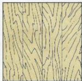
Random Match: No order or pattern is used when veneers are spliced.
