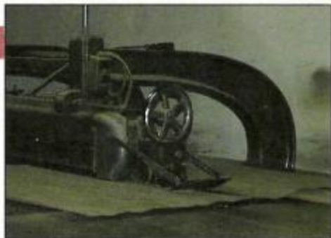
▲ A veneer splicer is used at the plywood plant to edge glue together pieces of flat-sliced veneer into a single sheet.
