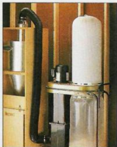
To connect a portable dust collector, run a flexible hose from the inlet of the vacuum to the cyclone.
