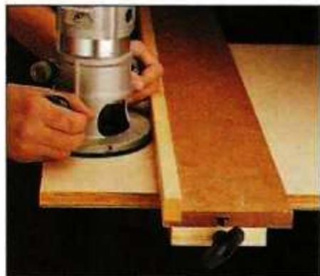
The fence doubles as a straightedge to guide the base of your router. Since the clamping system is beneath the guide, it won't get in the way of the motor housing.
