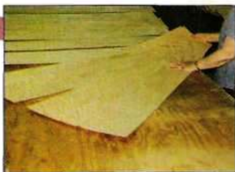
It's the selection of the face veneers at the factory that determines the grade of every sheet of hardwood plywood you buy.
