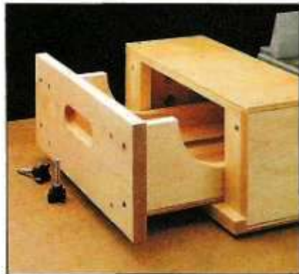
A. Wings: A pair of wings offer support to long stock and then "tuck" away inside the case for storage.
