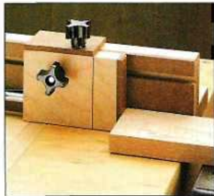
C. Stop System: For accurate repeat cuts, an adjustable stop slides in slots cut in the fence rails.
