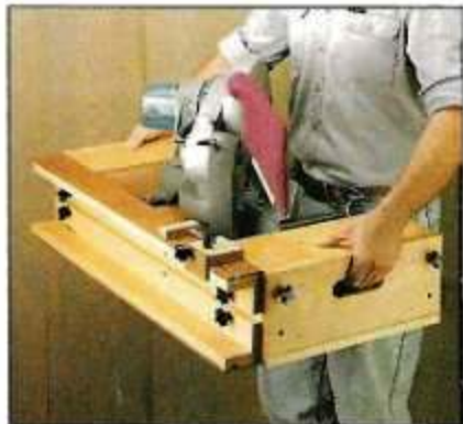
B. Portable: To make it easy to lift and carry the miter saw station, the wings have built-in handles.
