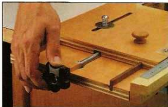
A straightedge makes it easy to set your router bit flush with the fence.
