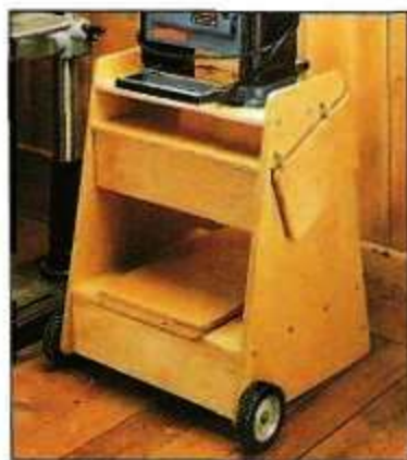
▲ The outfeed extension of the planer stand “knocks down” for moving and storage. The table lifts off and the “wings” fold back.
