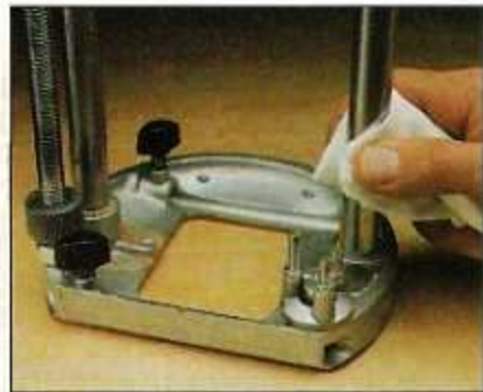
Plunge Tubes: Use a soft rag to clean the plunge tubes and rods. Then follow up the cleaning with a dry lubricant.
