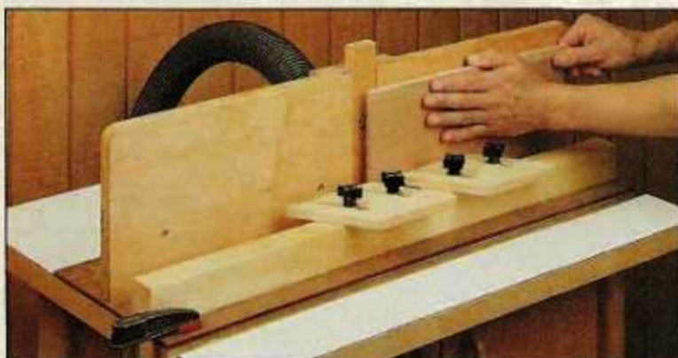
▲ To prevent chipout, a sliding insert forms a "zero-clearance" opening around the tip of the bit.
