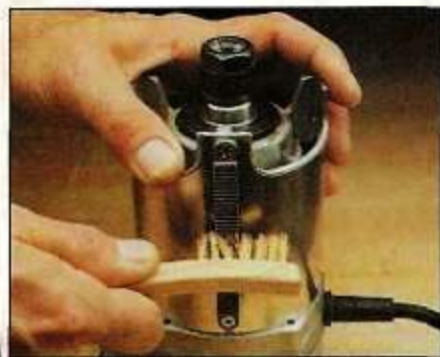
Rack and Pinion: I like to use a brass brush or an old toothbrush to clean the "teeth" on this type of height adjuster.
