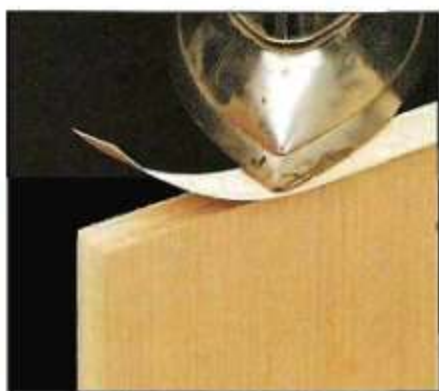
B. Iron-On Veneer. To glue this edging to the plywood, melt the layer of adhesive on the back with an ordinary iron.
