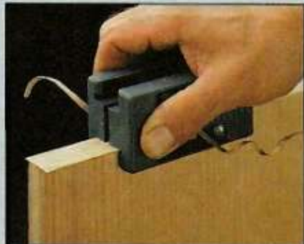
Double-Edge Trimmer. Spring-loaded sides on this trimmer adjust to the thickness of the plywood. Blades on each side remove both edges simultaneously.
