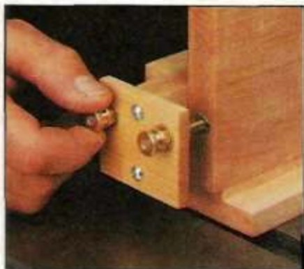
A. Micro-Adjustment System. A pair of knobs adjusts the jig to the desired size and spacing of the pins and slots.
