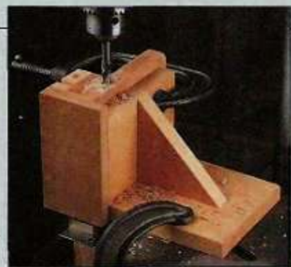
A vertical drilling jig holds long workpieces securely in place when drilling holes in end grain.
