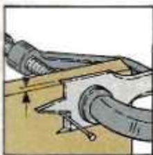
A nail and a scrap block lets you file an equal amount off both the edges of a spade bit.
