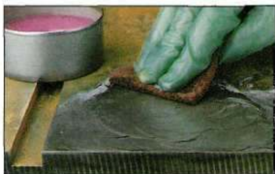
B. Rub in Chemical with Stripping Pad. A combination of a chemical dissolver like Naval Jelly and a furniture stripping pad removes the rest of the rust.
