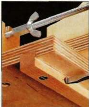
Adjustable Runner: Screws in the side of the runner allow you to adjust the fit to compensate for seasonal changes in humidity.
