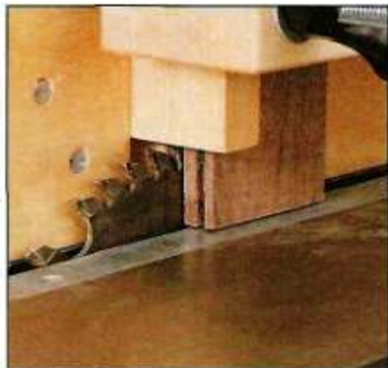
(B) Back Stop: The height of the back stop is adjustable to prevent the saw blade from cutting through it.
