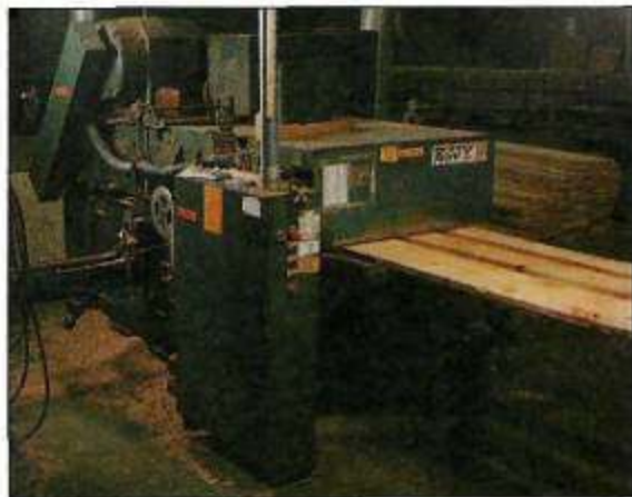
▲ Lumber mills and distributors use large planers to surface rough stock before it's sold. This removes the saw marks and leaves it uniform in thickness.
