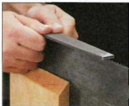
▲ Jointing: To ensure all the teeth on a saw are at the same height, a file is run lightly across the tips of the teeth.
