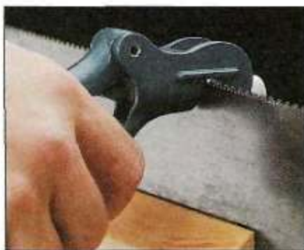
▲ Setting: Next, a tool called a saw set is used to bend the tips of the teeth. This keeps the blade from binding.
