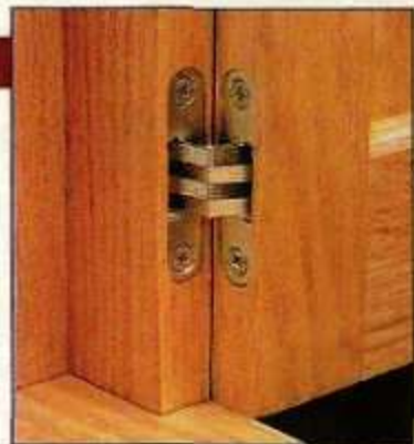
▲ The laminated links of this Soss Invisible Hinge slide inside the body. This conceals the hinge when it's closed.
