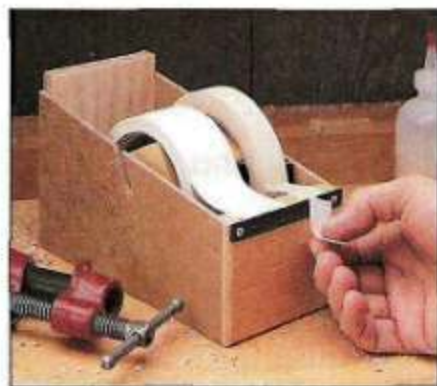
▲ This tape dispenser is another handy accessory. It's just a storage bin with a few modifications.
