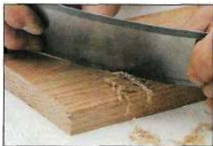
▲ Planer Marks. Hand scrapers can be used to quickly remove the ridges or marks left by a planer.
