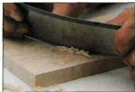
▲ Highly-Figured Grain. Smoothing highly-figured grain and burls is one area where a scraper has no equal.
