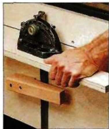
▲ A quick-access holder is mounted to the cabinet for your miter gauge. It allows you to slide the miter gauge in place — even with an auxiliary fence attached.
