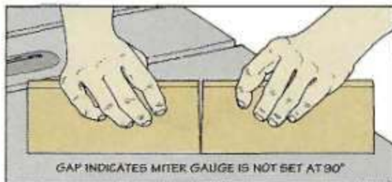
▲ Fig. 1. To check that your miter gauge is 90° to the blade, crosscut a piece of scrap. Flip one piece over and butt the cut ends together. If there's a gap the miter gauge needs to be adjusted.
