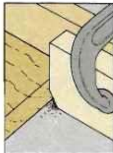
To prevent sawdust from building up between the workpiece and the stop block, cut a sawdust relief on the bottom corner.
