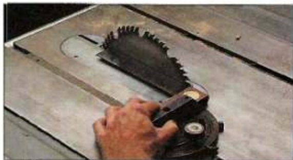
▲ Fig. 1. To check that your miter gauge is 90° to the blade, crosscut a piece of scrap. Flip one piece over and butt the cut ends together. If there's a gap the miter gauge needs to be adjusted.
