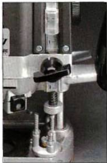
▲ A three position turret and a magnified hairline indicator allow for precise depth settings
