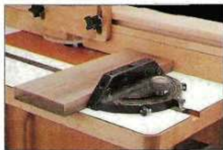
▲ A channel can be routed to accept your miter gauge. This is particularly handy for routing the ends of boards.
