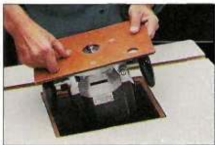
▲ The router is mounted to a removable insert plate so it can be lifted out for changing bits or free-hand routing.
