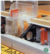
Rear view of table fence showing spring-tensioned fastenings
