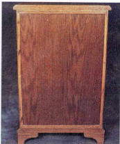
Rear detail of the router cabinet showing back panel pinned in to rebate
