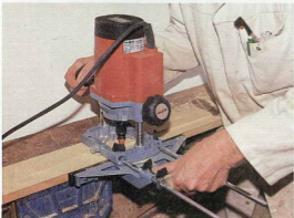
The side fence is essential when grooving
