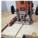
A home-made work aid is used for quick positioning of the initial cut
