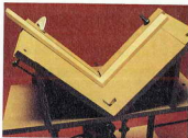
Note the support brackets clamped in place to help hold the workpiece in place
