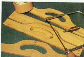
Cut just outside the pencil lines with a fret saw to produce the basic end piece
