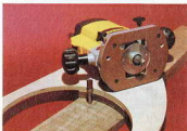
Position the template so the central lines on the template line up with the centre line on the post
