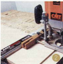
The first cut across a piece of Contiboard with the Accurate Guide fitted to the CMT 1E router
