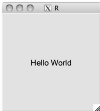
Figure 6.1: “Hello World” in GTK+. A window containing a single button displaying a label with the text “Hello World.”
