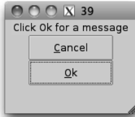
Figure 17.4: Simple GUI showing buttons with underline property. The underlined letters match bindings to the top-level window to invoke the button.
