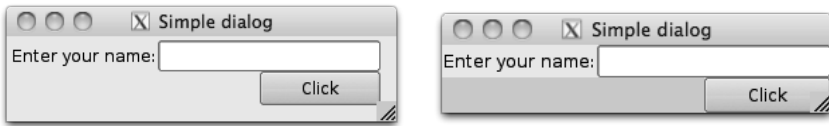
Figure 17.2: Comparison of themed versus non-themed dialogs. The non-themed one (right) one does not use an inner ttkframe , and in addition to not having padding, has mismatched colors.
