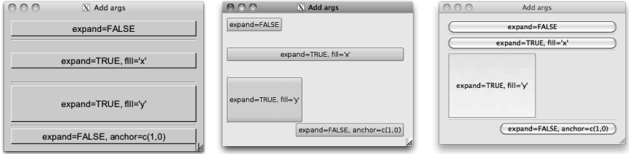
Figure 3.2: The expand , fill , and anchor arguments are implemented slightly differently in the different packages. ( gWidgetsRGtk2 on left, gWidgetstcltk in middle, and gWidgetsQt on right.). For GTK+, child components packed in a box container always fill in the direction opposite the packing, in this case the “x” direction. As such, the anchor directive has no effect. For tcltk a widget fills only if expand=TRUE is given. For gWidgetsQt expansion and fill are linked together.
