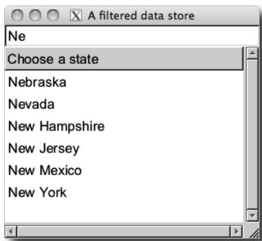
Figure 9.3: Example of a data model filtered by values typed into a text-entry widget.
