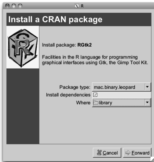
Figure 8.6: An installation wizard programmed using GtkAssistant. This is page four, which allows options for a call to install.packages to be configured.
