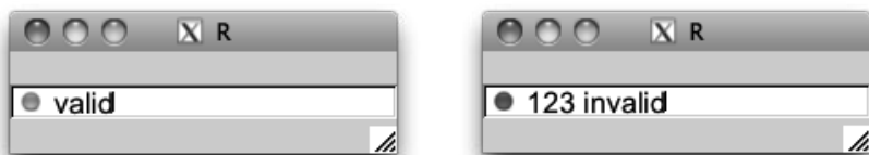
Figure 8.4: Illustration of adding an icon to a GtkEntry instance to indicate whether the text entered is valid.
